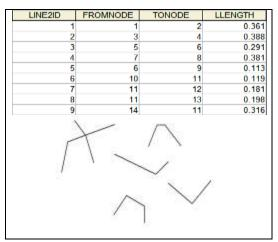
Figure 6: One-layer topology for line. **Region topology:** Running the software, creates an additional table i.e. three fields contain "Polygon nod", "Perimeter", and "Area", are added to an attributes table and one new table that contains three fields for representing topological relations. An instance of running software for this status has been represented in Figure 7.
