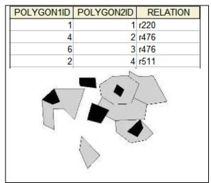
Figure 10: Inter-layer topology for polygon-polygon.
