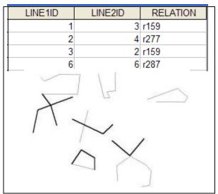
Figure 8: Inter-layer topology for line-line.
