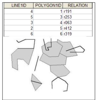
Figure 9: Inter-layer topology for line-polygon.
