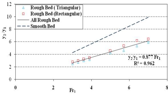
**Figure 5.** Relation between the depth ratio  $y_2/y_1$  and  $Fr_1$
