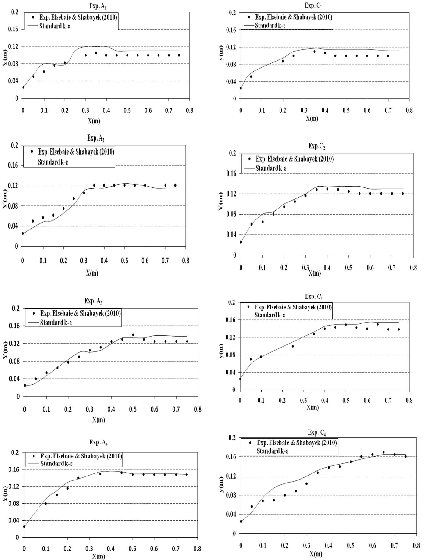
**Figure 4.** Comparison of free surface profiles between numerical turbulent models and experimental data
