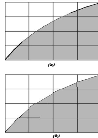
**Figure 1.** Interface calculations; (a) actual interface shape; (b) the geometric reconstruction scheme
