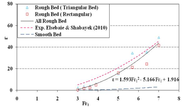
**Figure 7.** Comparison of shear force coefficient estimated from the turbulent model and experimental data
