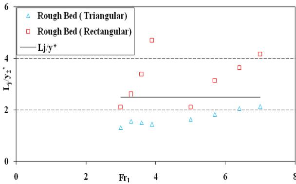
**Figure 6.** Relation between the ratio of  $L_j/y_2^*$  and  $Fr_1$
