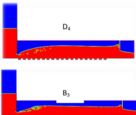
**Figure 3.** Simulation of water surface profiles using the VOF method for experiments D<sub>4</sub> and B<sub>3</sub>
