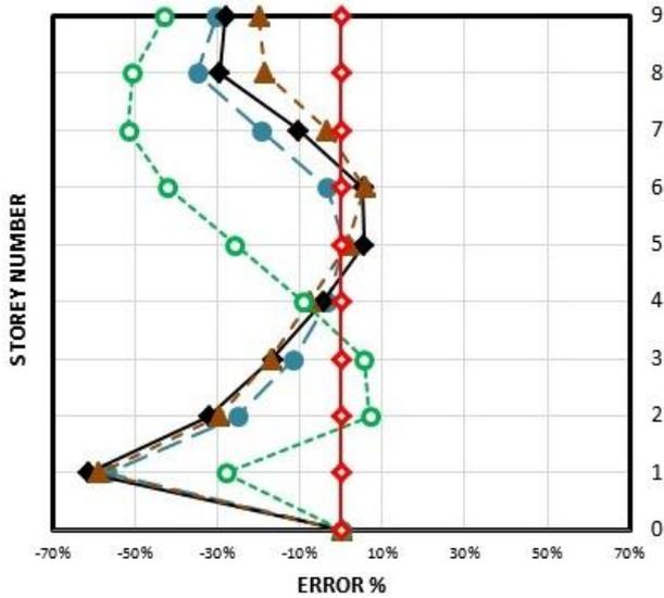
Figure 8. Predicted peak inter-story drift demands by NSPs compared to NTH analyses for 9-story SPSW building
