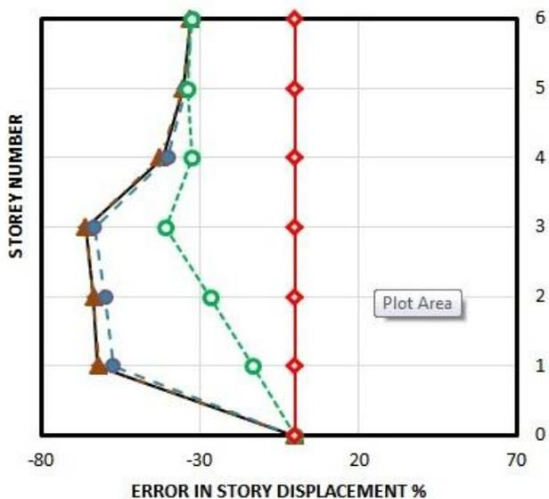
**Figure 6.** Predicted peak displacement demands and error accrued by NSPs compared to NTH analyses for 6-story SPSW building
