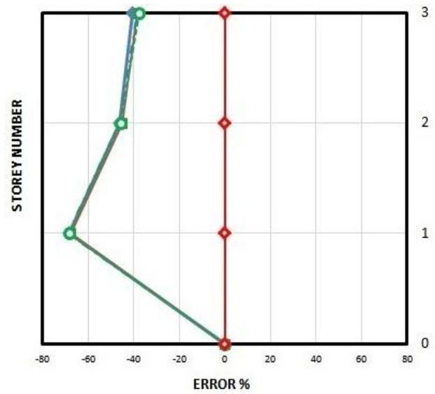
Figure 10. Predicted peak inter-story drift demands by NSPs compared to NTH analyses for 3-story SPSW building
