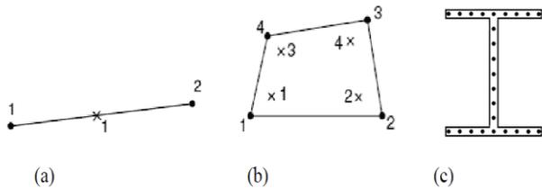
**Figure 3.** Integration point in (a) "B31" beam element and (b) "S4" shell element (c) I-shape cross section
