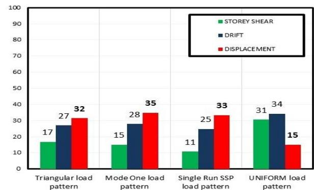
Figure 14. Comparison of the accuracy of the different NSPs parameters for 9-story SPSW building, using an error index defined by Eq. (9)
