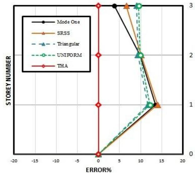
Figure 13. Predicted Shear Story by NSPs compared to NTH analyses for 3-story SPSW building
