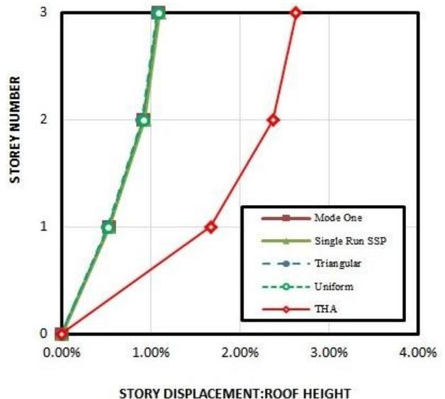
**Figure 7.** Predicted peak displacement demands and error accrued by NSPs compared to NTH analyses for 3-story SPSW building
