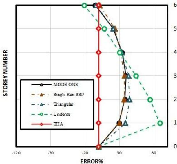
Figure 12. Predicted Shear Story by NSPs compared to NTH analyses for 6-story SPSW building
