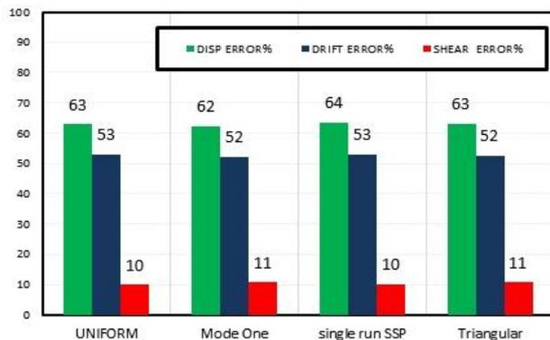
**Figure 16.** Comparison of the accuracy of the different NSP parameters for 3-story SPSW building, using an error index defined by Eq. (9)
