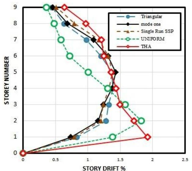
**Figure 8.** Predicted peak displacement demands and error accrued by NSPs compared to NTH analyses for 9-story SPSW building
