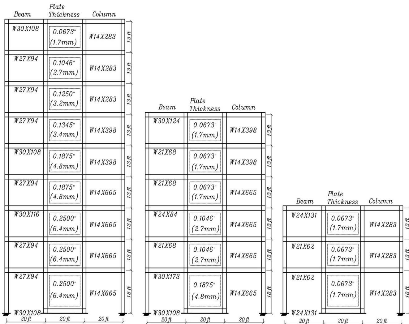
Figure 1. Dimensions and properties of SPSW building (Memarzadeh et al., 2011)
