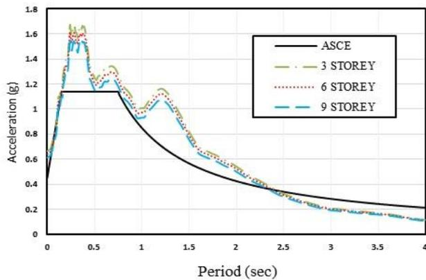
**Figure 4.** Scaled Response Spectra for each frames
