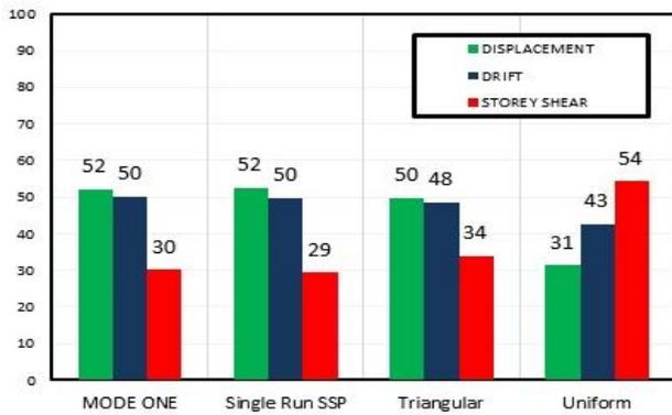
**Figure 15.** Comparison of the accuracy of the different NSP parameters for 6-story SPSW building, using an error index defined by Eq. (9)
