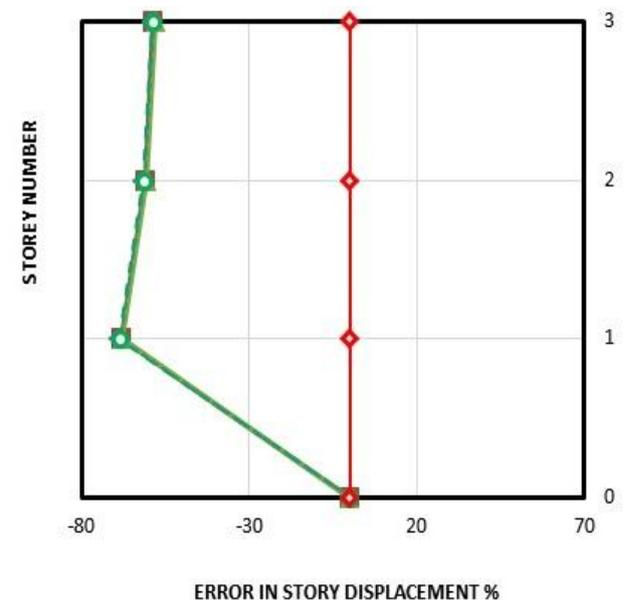
**Figure 7.** Predicted peak displacement demands and error accrued by NSPs compared to NTH analyses for 3-story SPSW building
