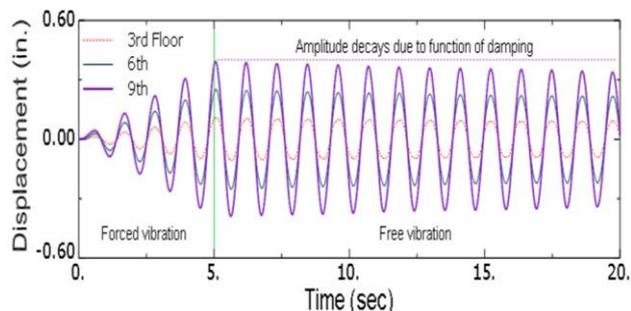
Figure 2. Lateral displacements of floors for 9 story SPSW (Memarzadeh et al., 2010)
