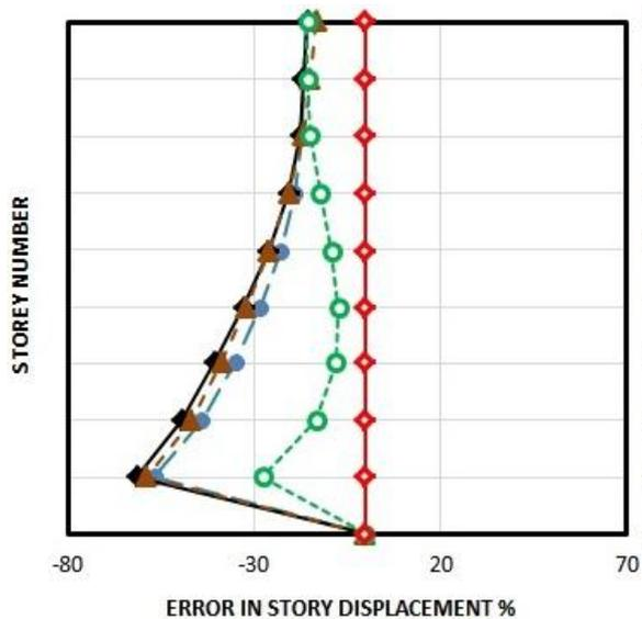
**Figure 5.** Predicted peak displacement demands and error accrued by NSPs compared to NTH analyses for 9-story SPSW building
