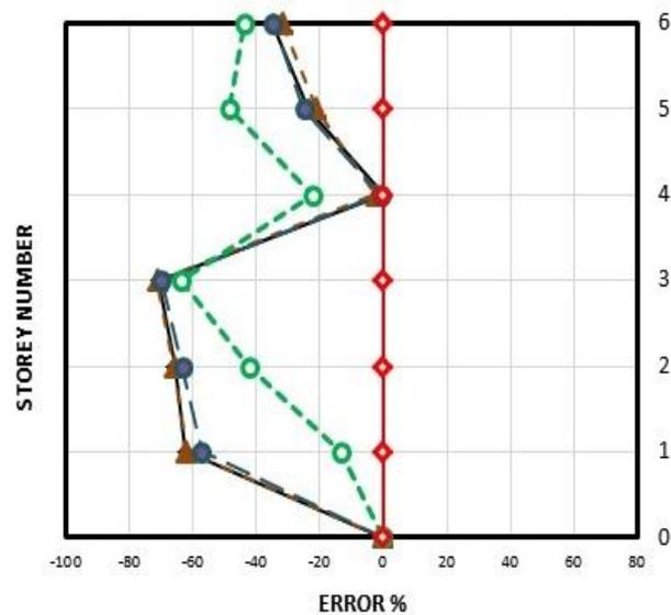
Figure 9. Predicted peak inter-story drift demands by NSPs compared to NTH analyses for 6-story SPSW building
