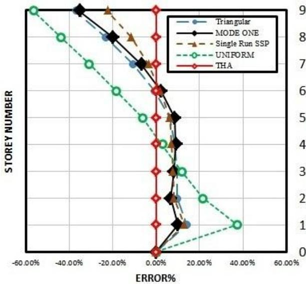
Figure 11. Predicted Shear Story by NSPs compared to NTH analyses for 6-story SPSW building
