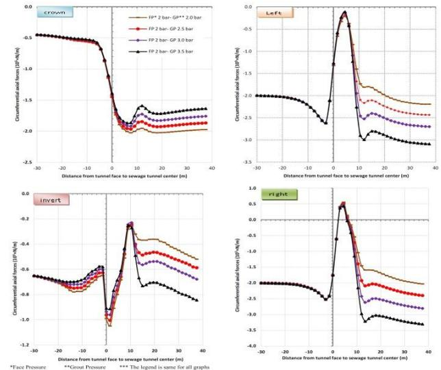
**Graph 4.** Variation of circumference axial force at the monitoring points when the face pressure is 2 bar and the grout pressure varies from 2 to 3.5 bar.
