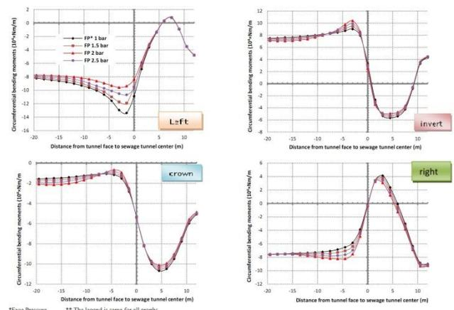
**Graph 1.** Variation of circumference bending moment at the monitoring points when the face pressure varies from 1 to 2.5 bar.
