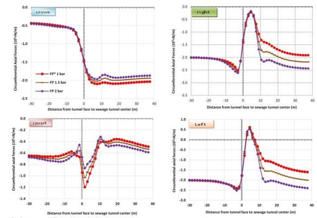
**Graph 2.** Variation of circumference axial force at the monitoring points when the face pressure varies from 1 to 2 bar.
