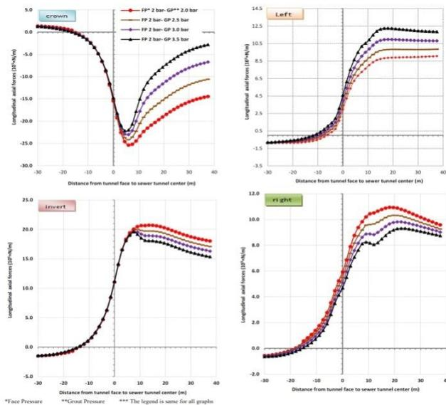
**Graph 6.** Variation of longitudinal axial force at the monitoring points when the face pressure is 2 bar and the grout pressure varies from 2 to 3.5 bar.
