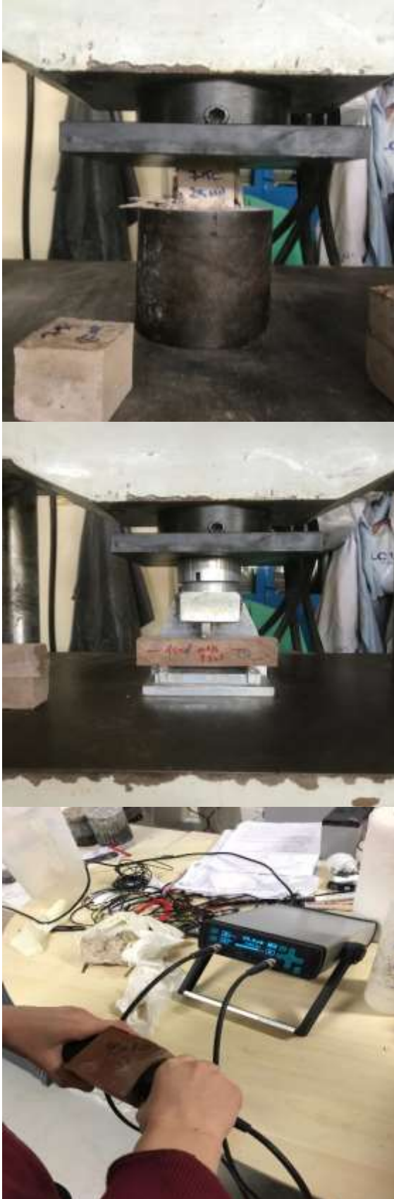
Figure 1. Compressive, flexural strength and ultrasonic pulse velocity test on samples.
