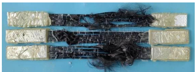
(b) Failure pattern
