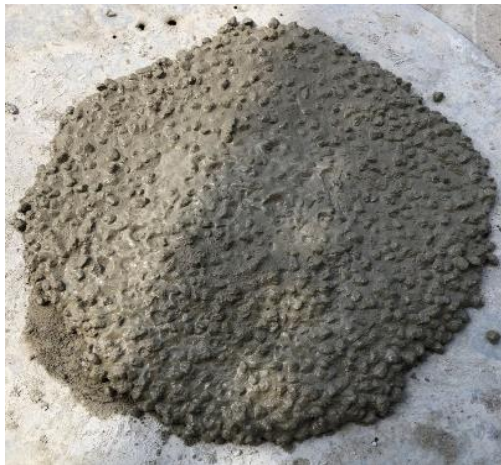
Figure 2. Slump flow of developed SCC
