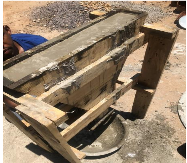
Figure 3. V-Funnel apparatus filled with fresh concrete.
