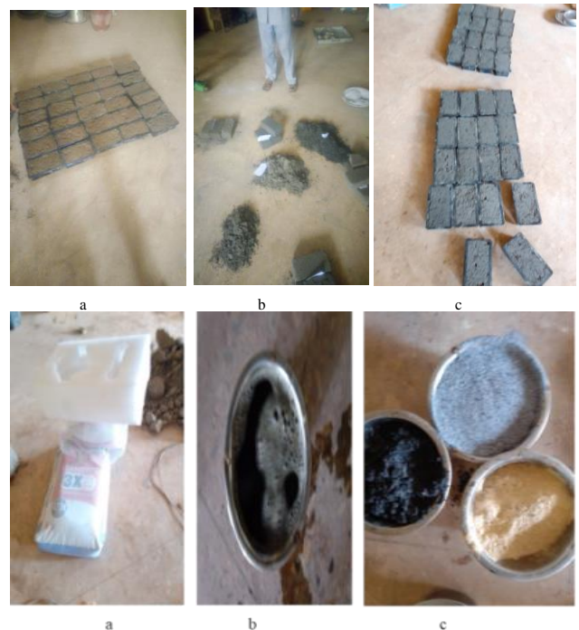
Figure 2. I= a) Geopolymer concrete using each binders and super plasticizer separately; b) Demolding of different geopolymer using each binders and super plasticizer after 48 hours casting, and c) geopolymer made using optimum values obtained from each binders. II= a) Cement; b) laboratory-created super plasticizer (from rice husk) and c) Fly ash, rice husk ash as well as kaolin clay.
