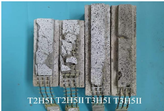
(a) CTRM strengthened concrete
