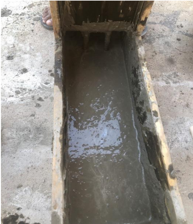
Figure 4 - L- box apparatus with SCC
