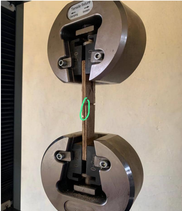
Figure 10a. glued joint between tensile loading jaw
