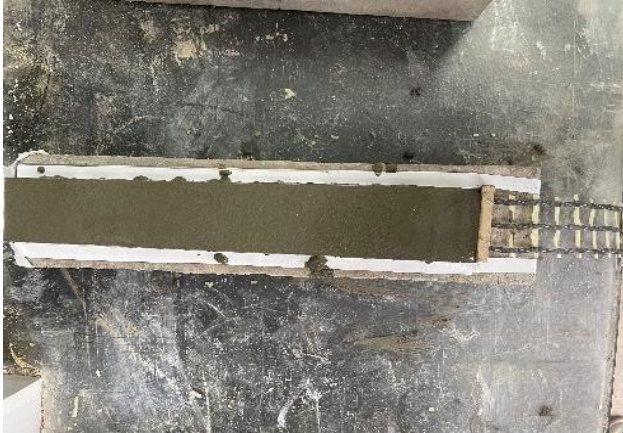
Figure 3. Preparation of CTRM strengthened concrete specimen
