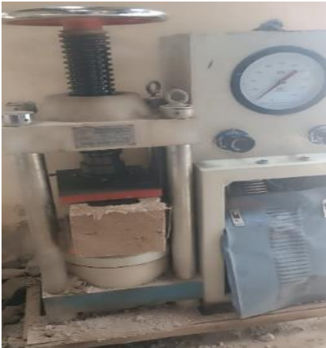
Figure 2. Compressive strength test
