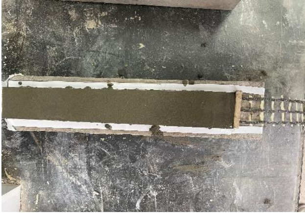
Figure 3. Preparation of CTRM strengthened concrete specimen
