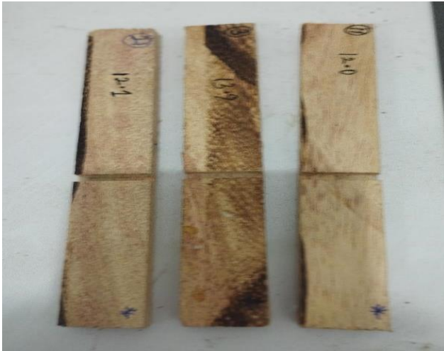
Figure 3. Resized, glued joints specimen.
