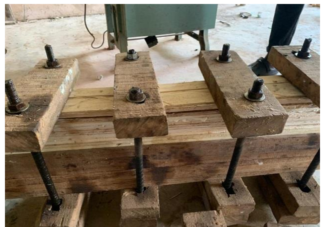
Figure 2. Clamping of laminates
