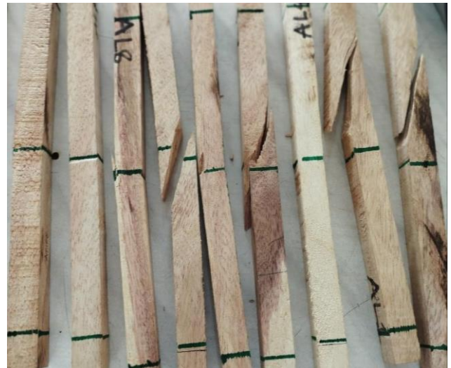
Figure 4: Samples after bending strength test
