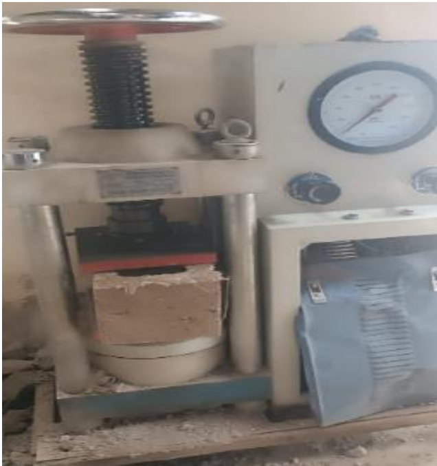
Figure 2. Compressive strength test
