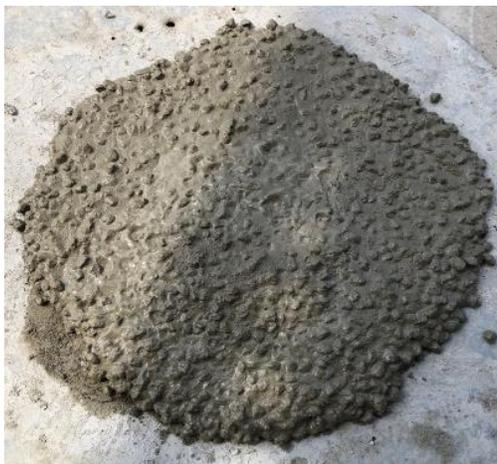
**Figure 2.** Slump flow of developed SCC
