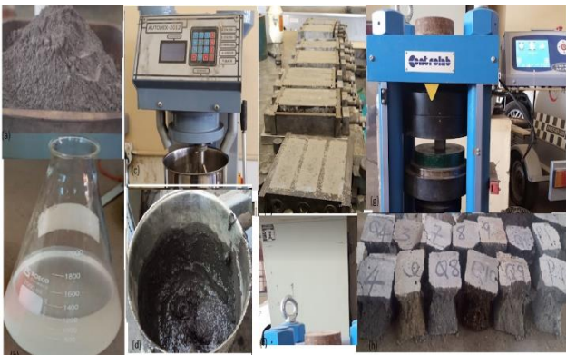
Figure 7. Production of geopolymer mortar
