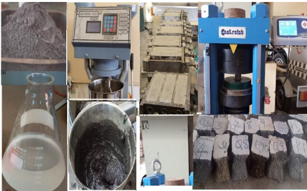
Figure 7. Production of geopolymer mortar
