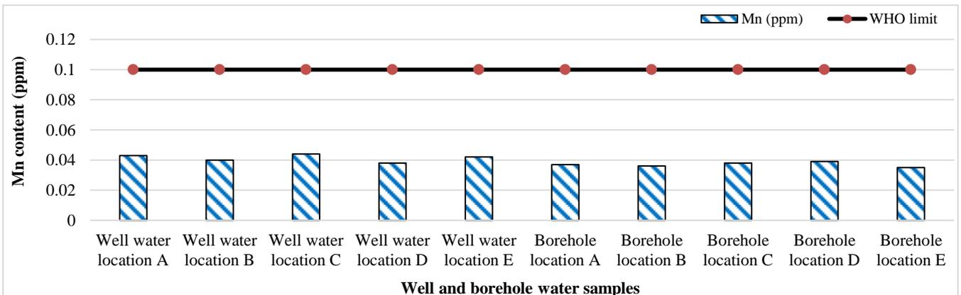
**Figure 4.** Mn content of well and borehole water samples
