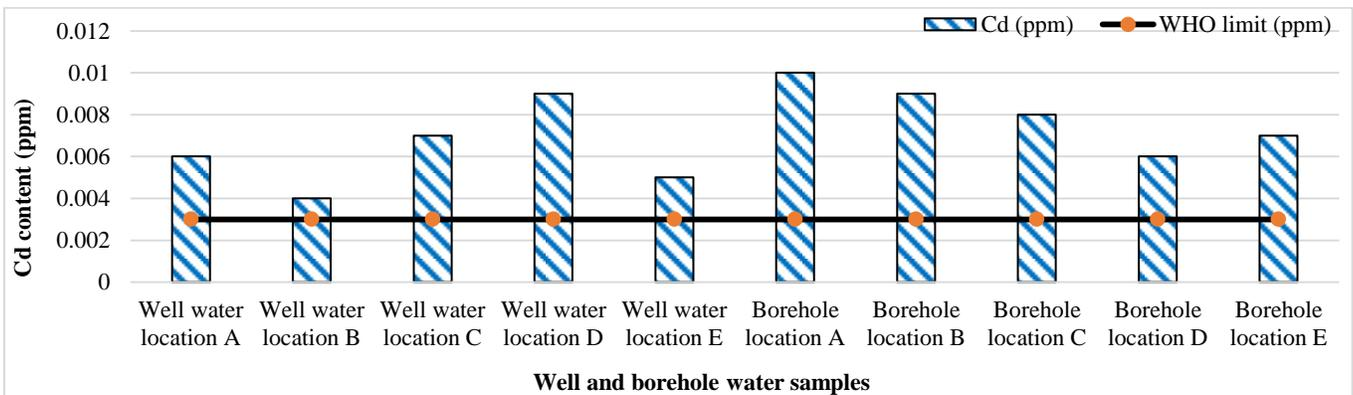
**Figure 3.** Cd content of well and borehole water samples
