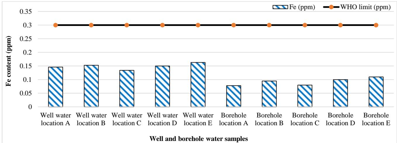
**Figure 1.** Fe content of well and borehole water samples
