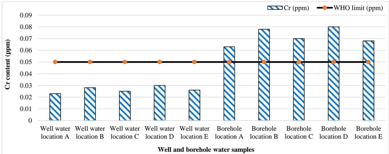
**Figure 2.** Cr content of well and borehole water samples
