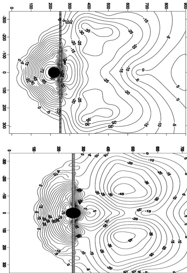
**Fig. 10.** Scour pattern for two cases (a)  $L=0$  and (b)  $L= -b/2$
