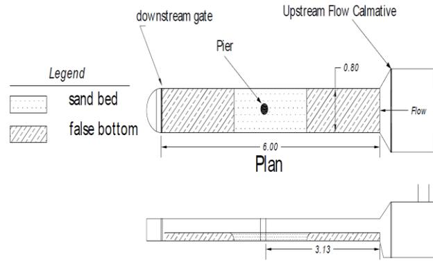
Figure 1. Flume - plan view and longitudinal profile
