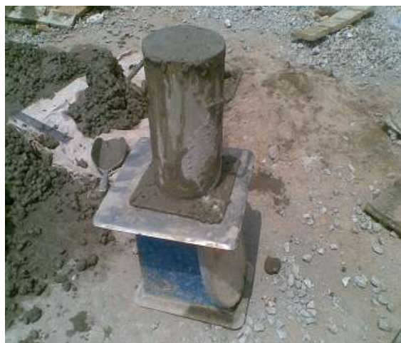
Figure 3. Concrete filled cylinder on weighing balance
