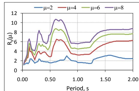
**Figure 22.** Strength reduction factor due to ductility for bilinear SDOF system with  $\alpha=0\%$  for Naghan earthquake
