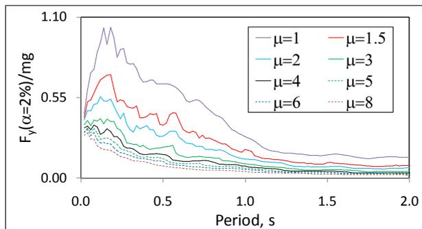
**Figure 8.** Mean inelastic strength demand spectra for bilinear SDOF system and  $\alpha=2\%$
