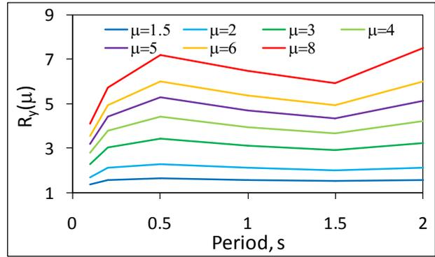
**Figure 16.** Regression values of response reduction factor due to ductility for bilinear SDOF system with  $\alpha=10\%$
