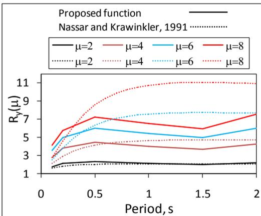
**Figure 19.** Comparison of proposed functional form for response reduction factor for bilinear SDOF system with  $\alpha=10\%$  and Nassar and Krawinkler [2]
