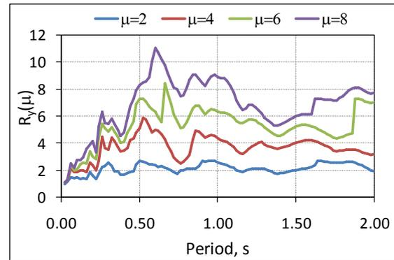
**Figure 20.** Strength reduction factor due to ductility for bilinear SDOF system with  $\alpha=0\%$  for El-Centro earthquake
