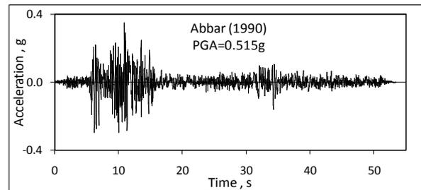
**Figure 4.** Abbar ground acceleration
