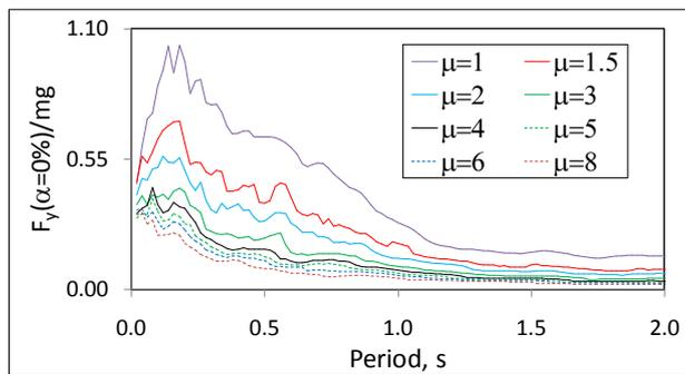
**Figure 7.** Mean inelastic strength demand spectra for bilinear SDOF system and  $\alpha=0\%$
