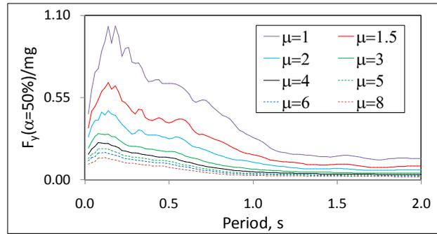
**Figure 10.** Mean inelastic strength demand spectra for bilinear SDOF system and  $\alpha=50\%$
