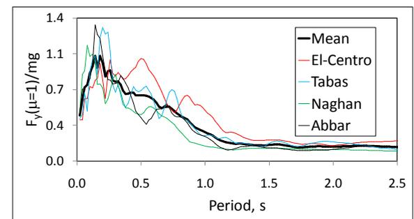
**Figure 5.** Scaled elastic response spectra of a bilinear SDOF system plus mean spectrum
