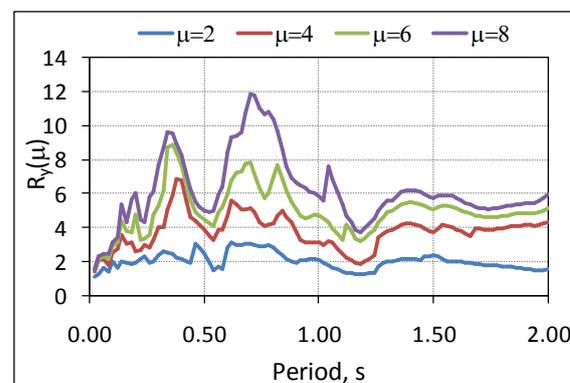
**Figure 23.** Strength reduction factor due to ductility for bilinear SDOF system with  $\alpha=0\%$  for Abbar earthquake
