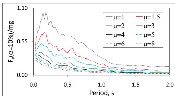
**Figure 9.** Mean inelastic strength demand spectra for bilinear SDOF system and  $\alpha=10\%$
