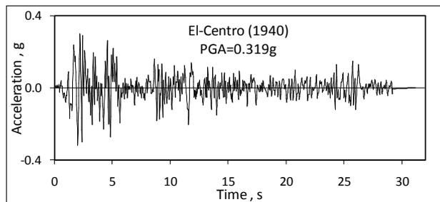
**Figure 1.** El-Centro ground acceleration
