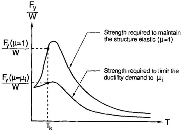
**Figure 14.** Linear and constant ductility nonlinear response spectra
