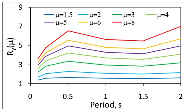
**Figure 15.** Regression values of response reduction factor due to ductility for bilinear SDOF system with  $\alpha=0\%$
