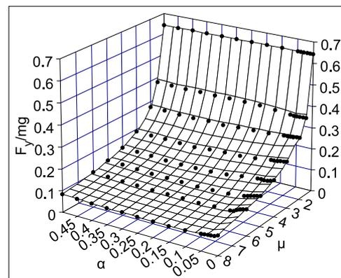
**Figure 12.** A 3D perspective view of the extracted points and the regressed surface at period of 0.5 seconds
