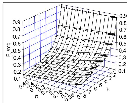
**Figure 11.** A 3D perspective view of the extracted points and the regressed surface at period of 0.1 seconds
