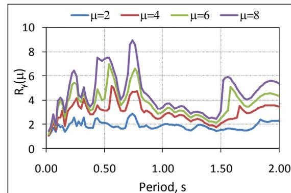
**Figure 21.** Strength reduction factor due to ductility for bilinear SDOF system with  $\alpha=0\%$  for Tabas earthquake
