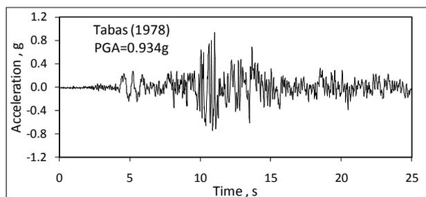
**Figure 2.** Tabas ground acceleration
