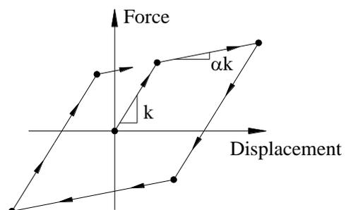
**Figure 6.** Bilinear hysteretic model used in this study
