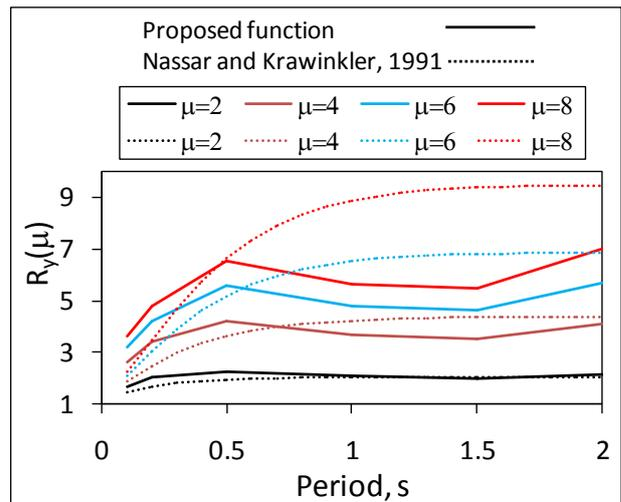
**Figure 17.** Comparison of proposed functional form for response reduction factor due to ductility for bilinear SDOF system with  $\alpha=0\%$  and Nassar and Krawinkler [2]
