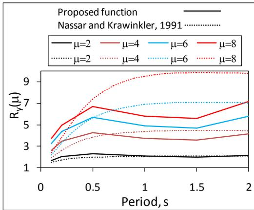
**Figure 18.** Comparison of proposed functional form for response reduction factor for bilinear SDOF system with  $\alpha=2\%$  and Nassar and Krawinkler [2]
