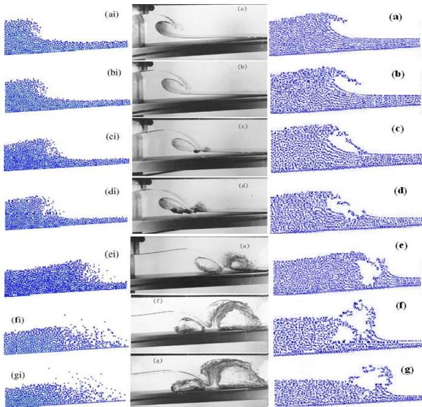
**Figure 6.** Qualitative comparison of laboratory photographs (center) with ISPH (right) (Khayyer et al., 2008) and WCSPH (left) snapshots.
