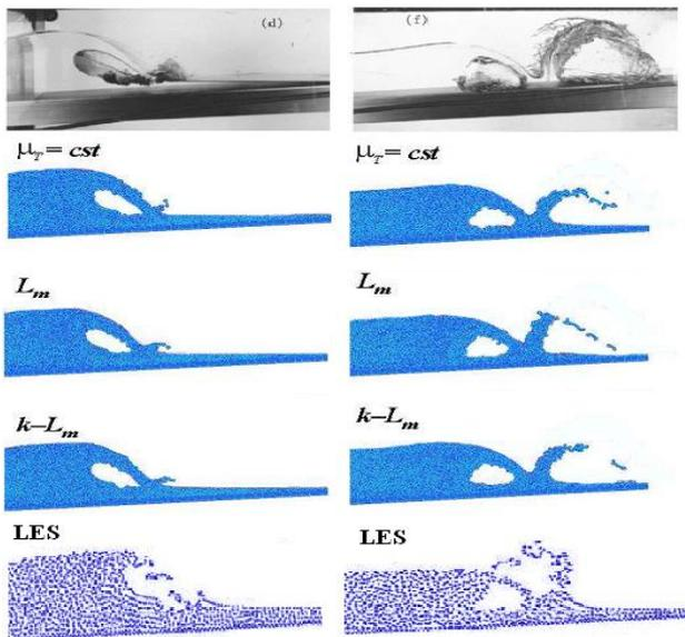
**Figure 4.** Qualitative comparison of laboratory photographs (Li and Raichlen, 2003) with simulated one achieved by SPH with various turbulence models (Issa and Violeau, 2009) and LES model (present study) at the initial step of the splash up process.
