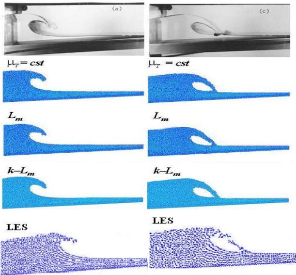
**Figure 3.** Qualitative comparison of laboratory photographs (Li and Raichlen, 2003) with simulated one achieved by SPH with various turbulence models (Issa and Violeau, 2009) and LES model (present study) at the initial steps of the plunging wave process.
