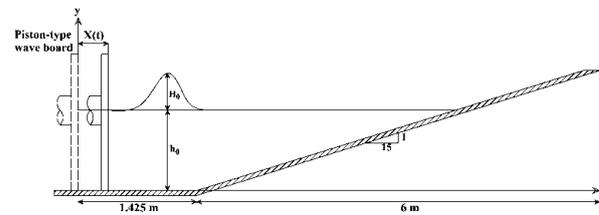
**Figure 1.** Computational domain for simulation of solitary wave breaking.
