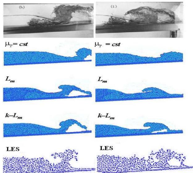
**Figure 5.** Qualitative comparison of laboratory photographs (Li and Raichlen, 2003) with simulated one achieved by SPH with various turbulence models (Issa and Violeau, 2009) and LES model (present study) at the final stages of splash-up
