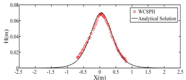
**Figure 2.** Comparison between the simulated and analytical wave profile for  $h_0 = 0.2$  m and  $H_0 = 0.07$  m.
