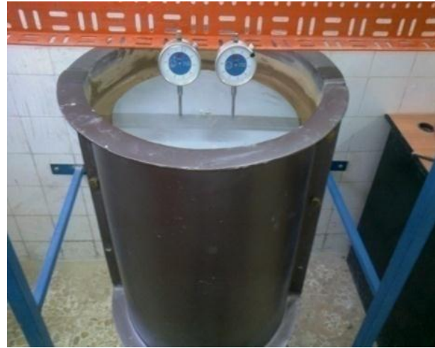
Figure 11. Plate of (GPA-Foundation System) under the Heave
