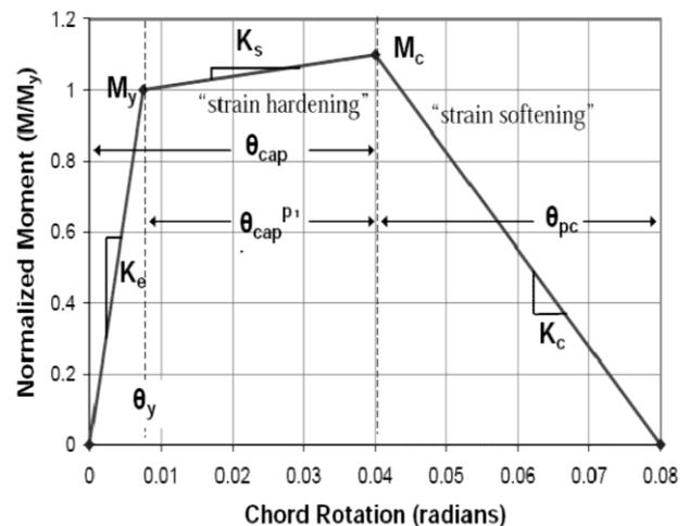
Figure 2. Monotonic behavior of an RC component (Ibarra et al., 2005)
