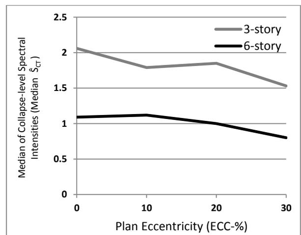
**Figure 6b.** Median of collapse spectral intensities ( $\hat{S}_{CT}$ ) vs. plan eccentricity ratio for 3 and 6-story models (Z direction)
