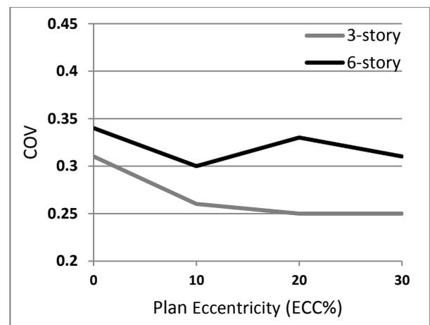
**Figure 7a.** Comparison of COV values for 3 and 6-story models (X direction)
