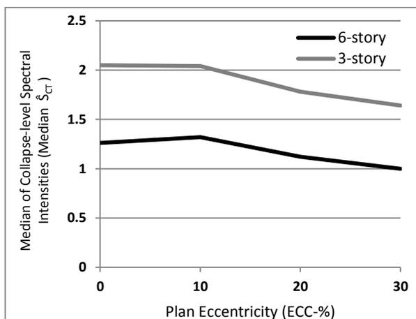
**Figure 6a.** Median of collapse spectral intensities ( $\hat{S}_{CT}$ ) vs. plan eccentricity ratio for 3 and 6-story models (X direction)
