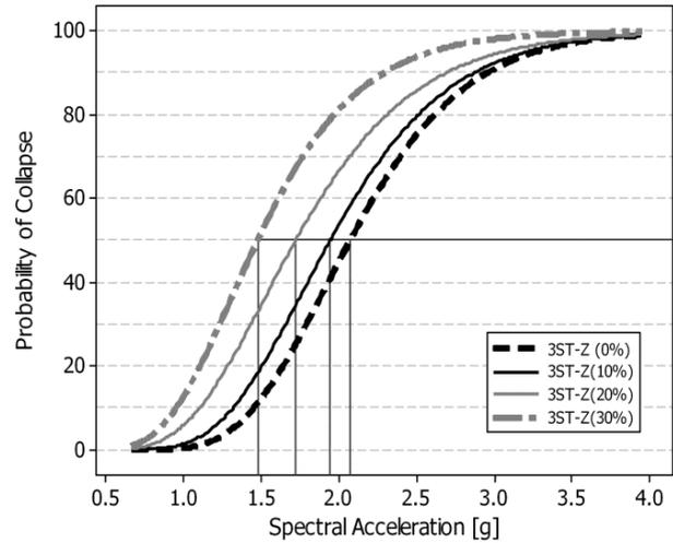
**Figure 8b.** CDFs (Fragility curves) for the 3-story model with different eccentricities (Z-Direction)
