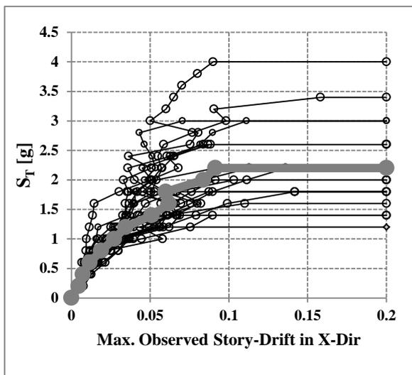
**Figure 5a.** IDA curves with the median curve (3-story model; X-Dir; ECC: 0%)
