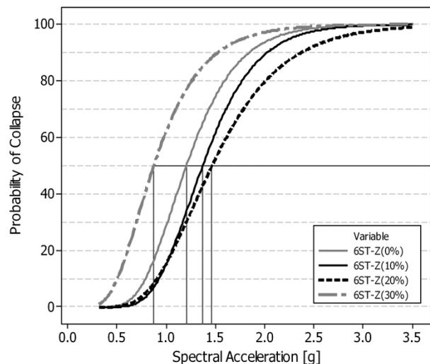
**Figure 9b.** CDFs (Fragility curves) for the 6-story model with different eccentricities (Z-direction)
