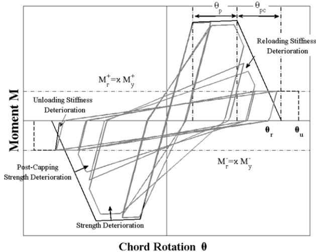
**Figure 3.** Hysteretic response of RC elements with stiffness and strength degradation (Ibarra et al., 2005)
