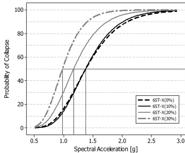
**Figure 9a.** CDFs (Fragility curves) for the 6-story model with different eccentricities (X-direction)
