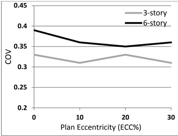
**Figure 7b.** Comparison of COV values for 3 and 6-story models (Z direction)
