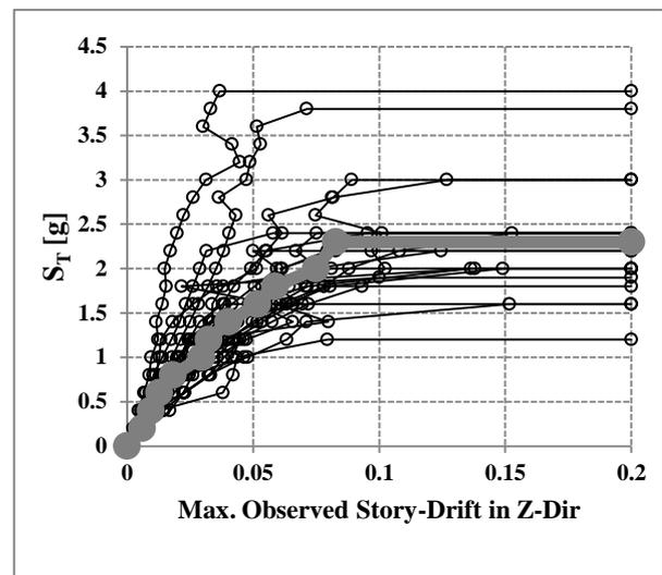
**Figure 5b.** IDA curves with the median curve (3-story model; Z-Dir; ECC: 0%)
