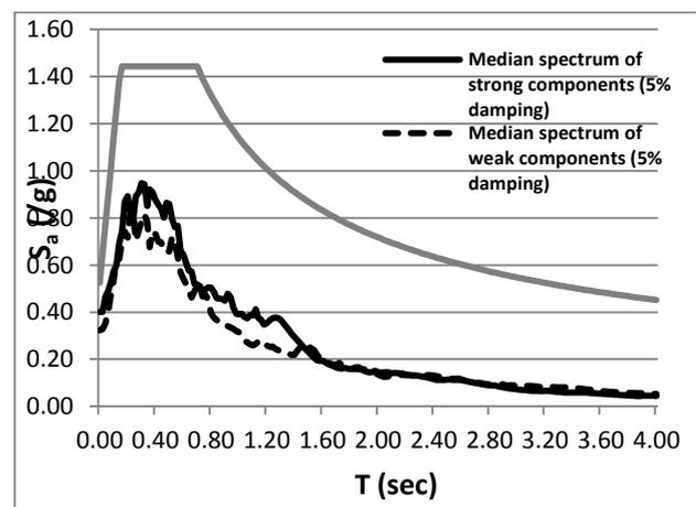
**Figure 4.** Median spectrum of strong and weak components of records with the design MCE level spectrum
