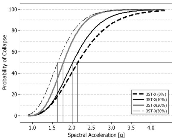
**Figure 8a.** CDFs (Fragility curves) for the 3-story model with different eccentricities (X-direction)
