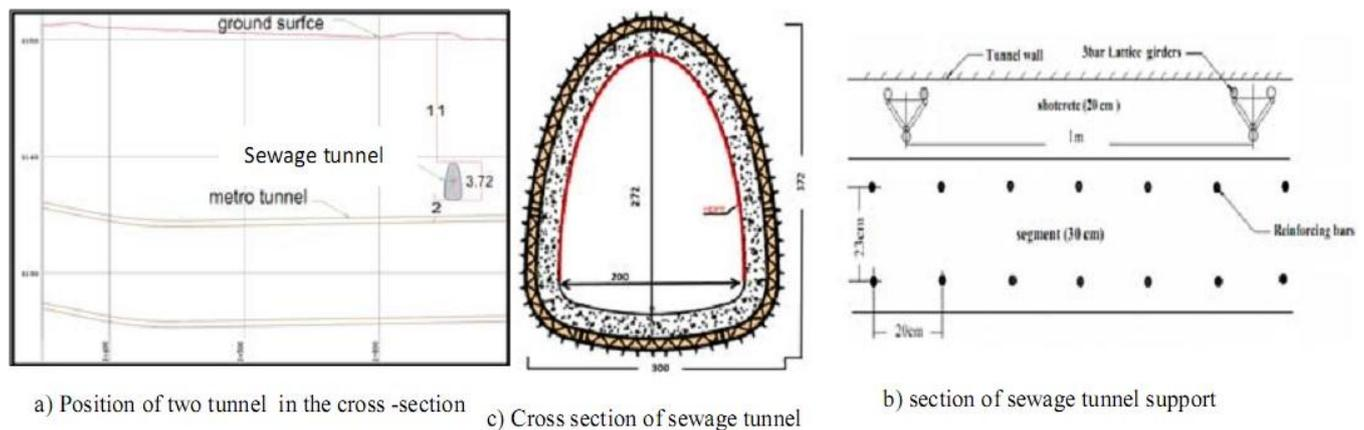
**Figure 1.** Geometry and position of sewage tunnel
