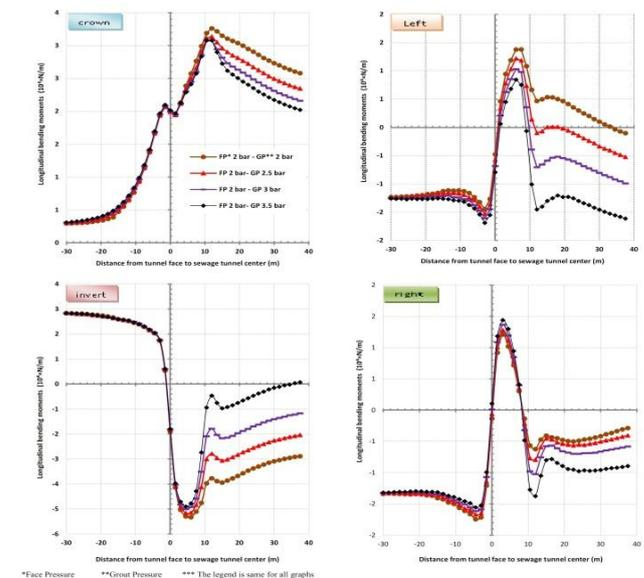
**Graph 5.** Variation of longitudinal bending moment at the monitoring points when the face pressure is 2 bar and the grout pressure varies from 2 to 3.5 bar.
