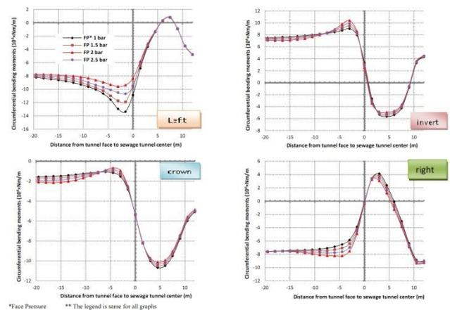
**Graph 1.** Variation of circumference bending moment at the monitoring points when the face pressure varies from 1 to 2.5 bar.
