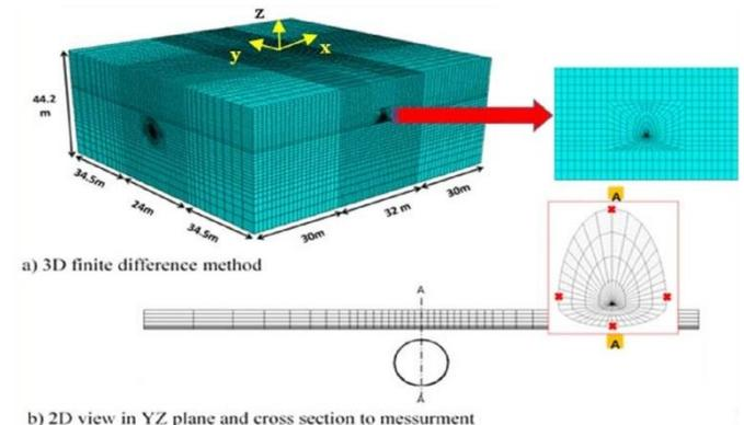
**Figure 2.** Finite difference model and cross section to measurement
