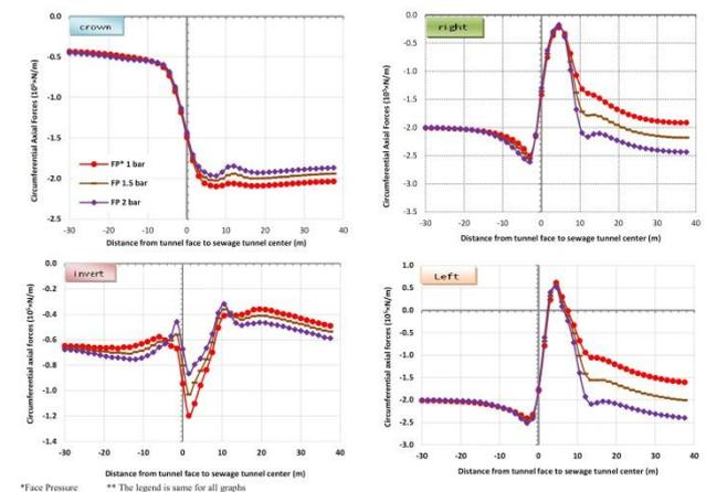
**Graph 2.** Variation of circumference axial force at the monitoring points when the face pressure varies from 1 to 2 bar.
