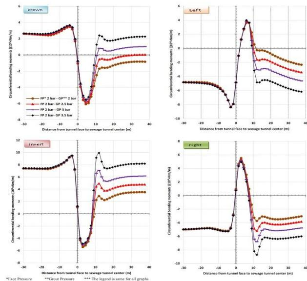
**Graph 3.** Variation of circumference bending moment at the monitoring points when the face pressure is 2 bar and the grout pressure varies from 2 to 3.5 bar.
