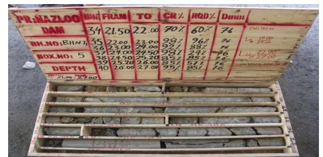
Figure 3. A view of barehole discovery box named BHNT 1 which was placed in 21 to 27 depths.
