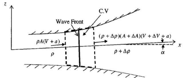
**Figure 1.** Control volume diagram used for continuity equation derivation
