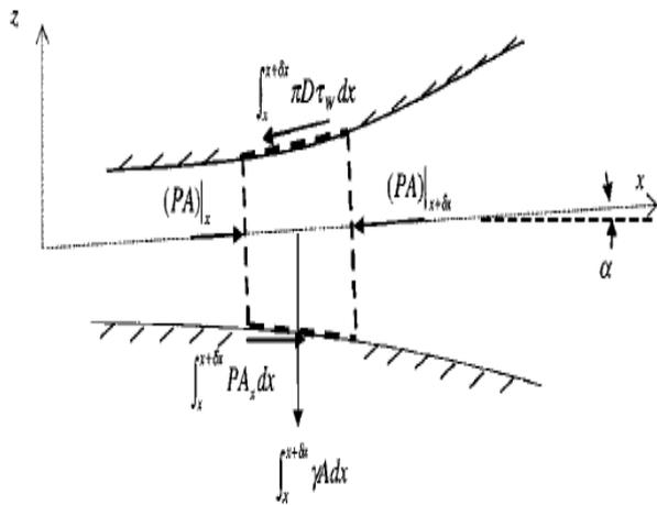
**Figure 2.** Control volume diagram used for momentum equation derivation
