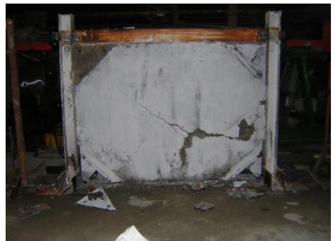
Figure 13. The second sample breakage manner
