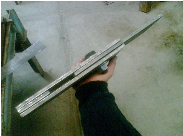
Figure 14. An image of the applied frictional sliding fuse
