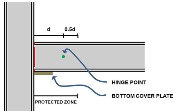
Figure 3. Protected zone for Full welded moment connection ( $d$ = beam depth)
