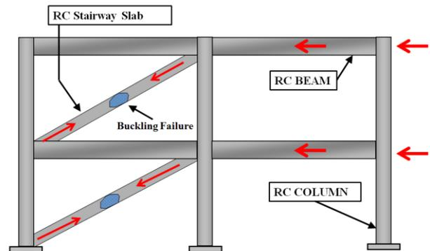
**Figure 6.** Stairway-Frame interaction failure potentialities
