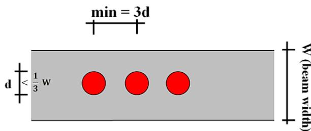
**Figure 4.** ACI 318-11 pipe and sleeve placing requirements (top RC beam view)
