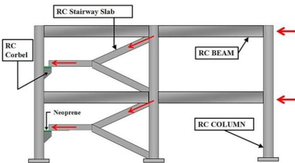
**Figure 18.** RC sliding corbel connection for interaction removal
