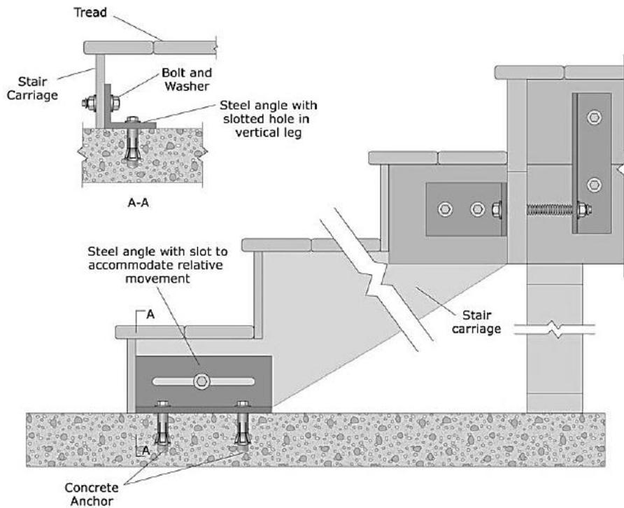
**Figure 7.** Stairway with landing with single run between (FEMA E-74, 2011)
