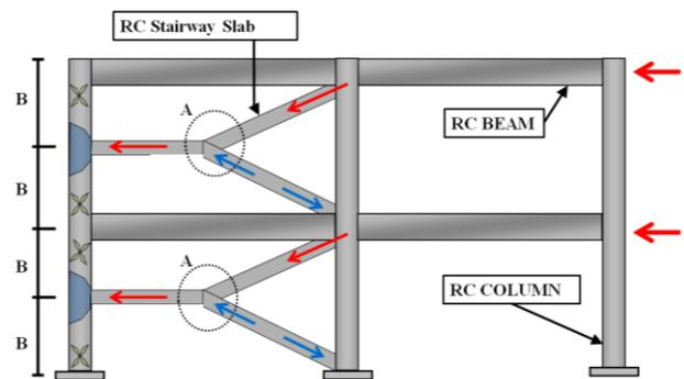
**Figure 5.** Stairway-Frame interaction failure potentialities
