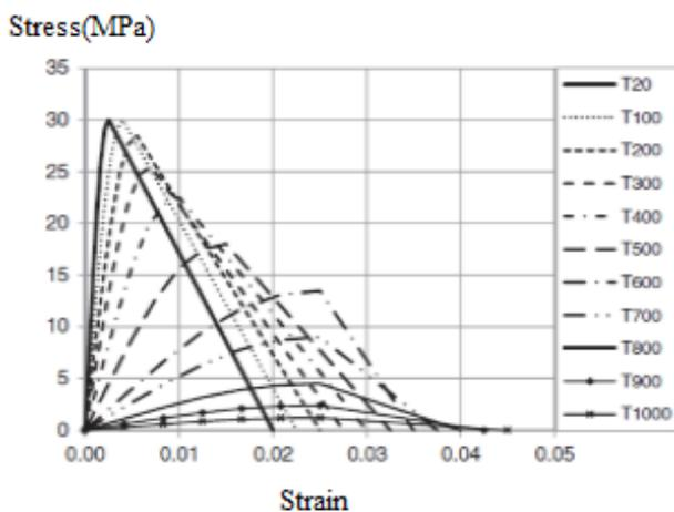
Figure 5. Stress-strain curve of concrete affected by heat increase
