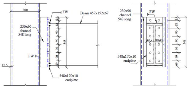
Figure 9. Connection with extensive endplate
