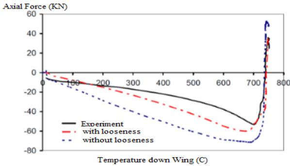
**Figure 17.** Comparison of beam axial load with looseness of different screw
