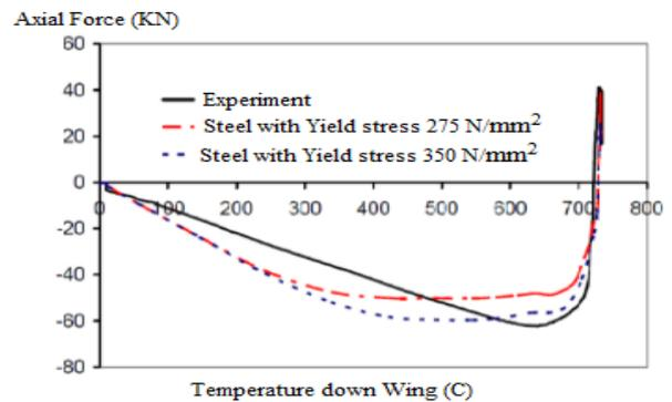
Figure 15. Comparison of axial force of beam with various yield stress
