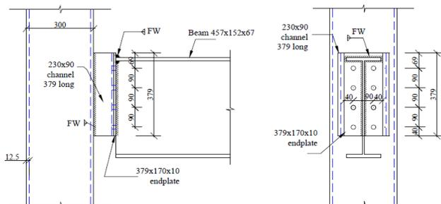
Figure 10. Connection with flexible balanced endplate
