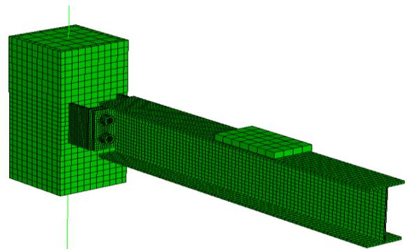
Figure 12. Connection finite element model
