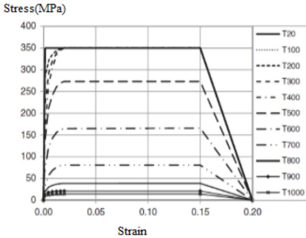
Figure 4. Stress-strain curve of steel under the effect of heat increase
