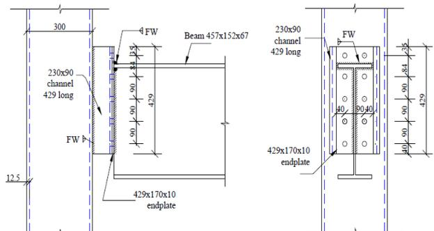
Figure 11. Connection with flexible extensive endplate
