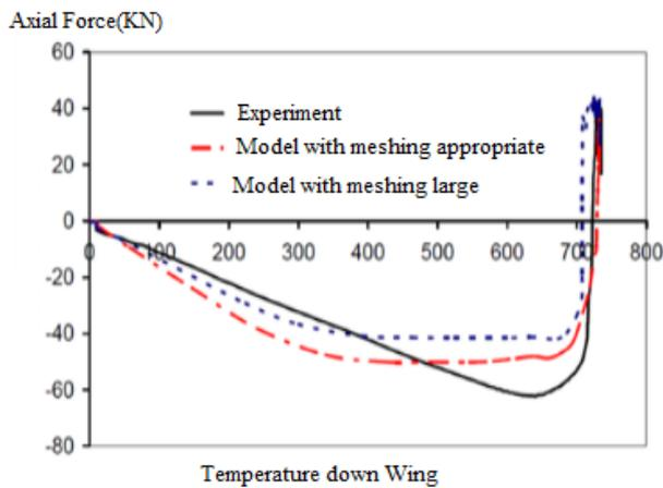
Figure 13. Comparison of axial force of beam by various mesh classification
