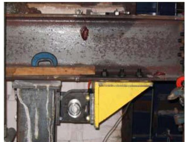
**Figure 3.** The clamped scheme of end of column in Wang and Ding's test
