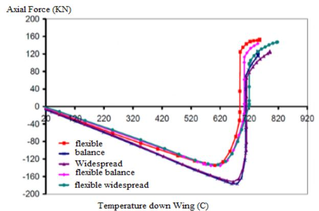
**Figure 21.** Comparison of beam axial force in connections with different endplate
