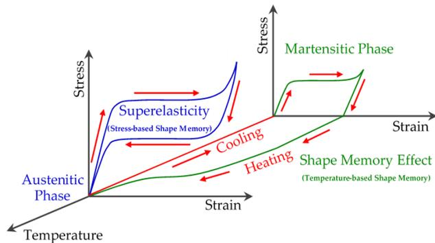
**Figure 1.** The schematic representation of shape memory effect and superelasticity of SMA materials
