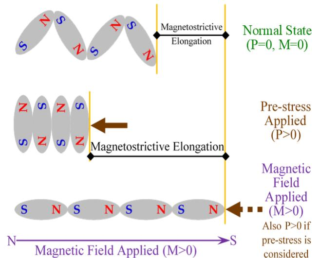
**Figure 11.** Schematic representation of the magnetostrictive effect (normal state and pre-stress added) described by the ellipsoid model.
