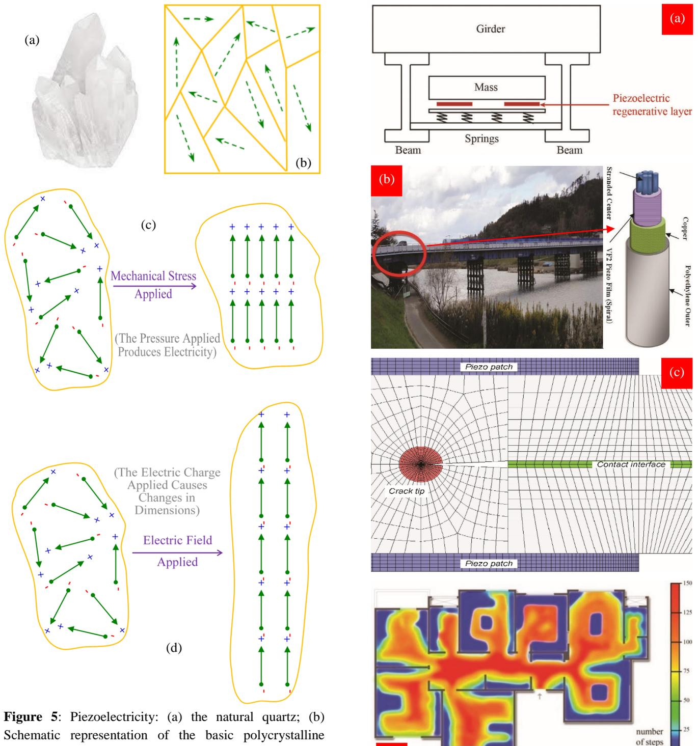
**Figure 5:** Piezoelectricity: (a) the natural quartz; (b) Schematic representation of the basic polycrystalline structure with the random polar axes; (c) the direct piezoelectric effect; (d) the inverse piezoelectric effect
