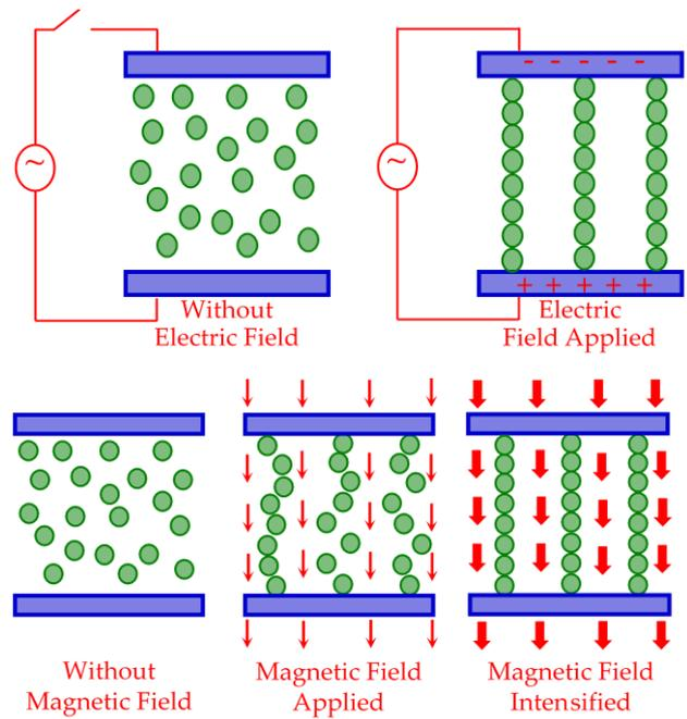
**Figure 8:** Schematic representations of the arrangement of the suspended particles in ER (up) and MR (down) fluids, subjected to respectively electric and magnetic fields
