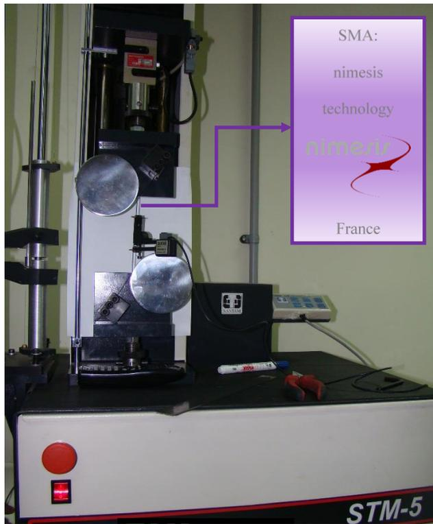
**Figure 13:** Experimental verification of the suitability of SMAs for structural earthquake engineering applications: (up) the test apparatus; (down) the superelastic behavior exhibited by the tested SMA wire under cyclic loading
