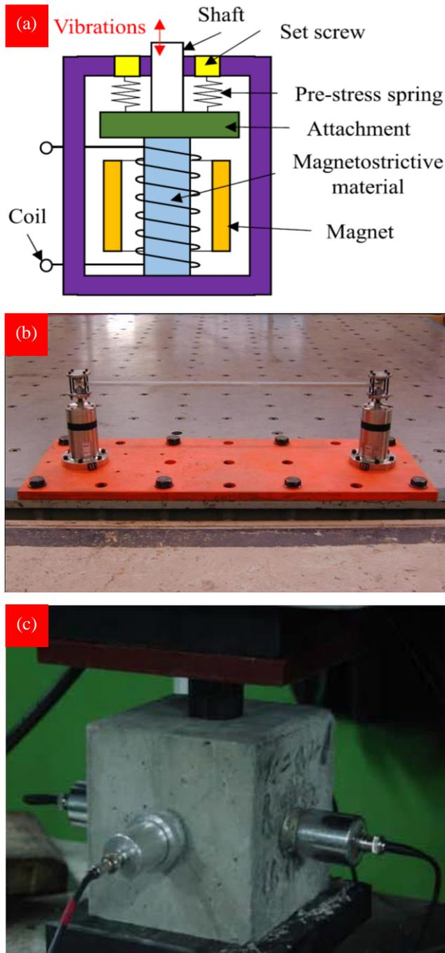
**Figure 12.** Civil engineering applications of the magnetostrictive materials: (a) schematic of a magnetostrictive actuator (Deng and Dapino, 2018); (b) vibration control of a beam (Moon et al., 2005); (c) non-destructive evaluation (Dong et al., 2011)
