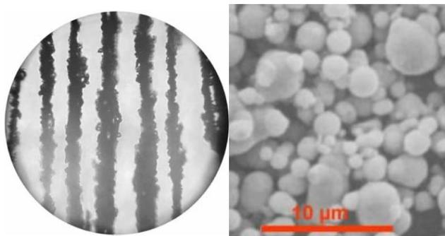
**Figure 7:** The micrograph of a MR fluid subjected to magnetic field (left), compared with the micrograph of the fluid without magnetic field (Spaggiari, 2013)
