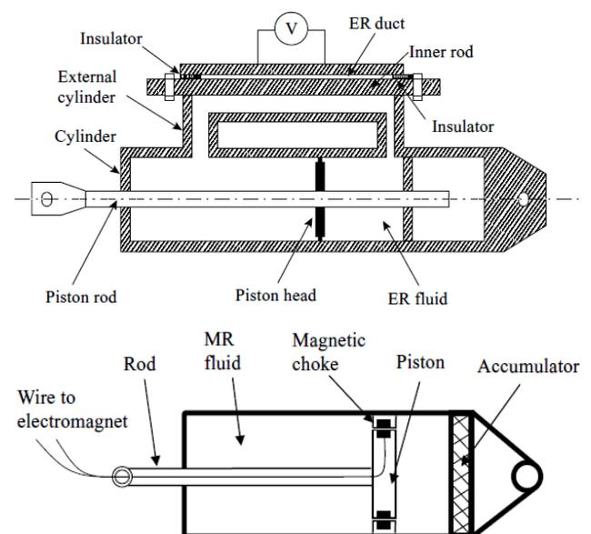
**Figure 9:** Schematics of ER (up) and MR (down) dampers (Cheng et al., 2008), representing the working principles of these two smart dampers
