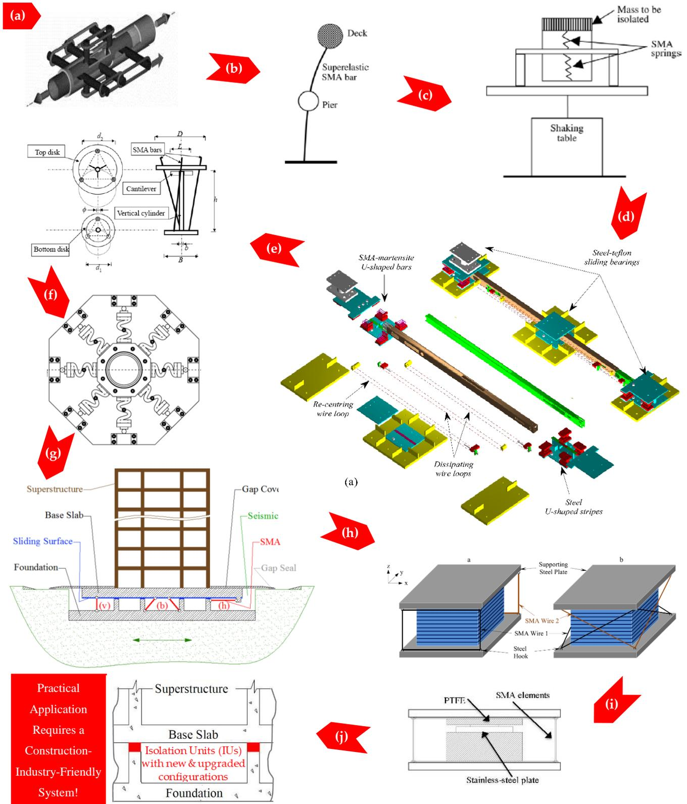
**Figure 3.** The SMA-based aseismic isolation systems: (a) Dolce et al (2000); (b) Wild et al. (2000); (c) Khan and Lagoudas (2002); (d) Cardone et al. (2003); (e) Casciati et al (2007); (f) Attanasi et al. (2008); (g) Cardone et al. (2009); (h) Hedayati Dezfuli and Shahria Alam (2013); (i) Ozbulut and Silwal (2014); (j) Narjabadifam (2015).
