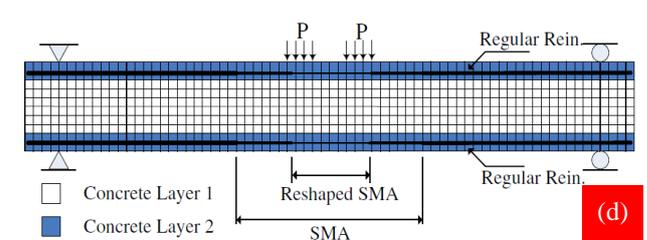
**Figure 2.** Civil engineering applications of SMAs in the forms of (a) martensitic beam-column connections (Ocel et al., 2004), (b) austenitic beam-column connections (Moradi and Shahria Alam, 2015), (c) braces (Qiu and Zhu, 2017), and (d) rebars (Abdulridha et al., 2013).
