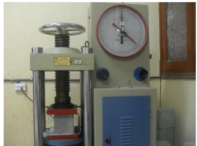
Figure 2. Hydraulic pressure machine used for compressive strength test
